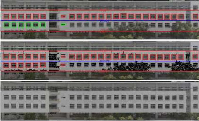
Figure 7. Result of occlusion removal and mending.
