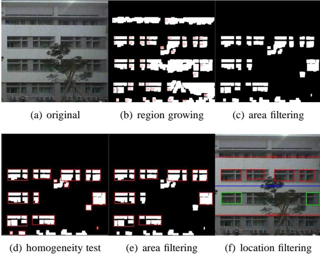
Figure 6. Procedure of self-mending facade occlusions.
