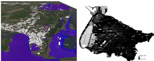
Figure 15. Potential flood perils of a 200-year frequency flood modeling.
