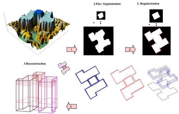
Figure 3. Building reconstruction from LIDAR data.
