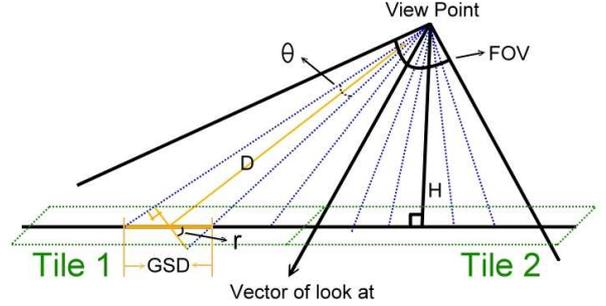
Figure 8. Ground sample distance (GSD).
