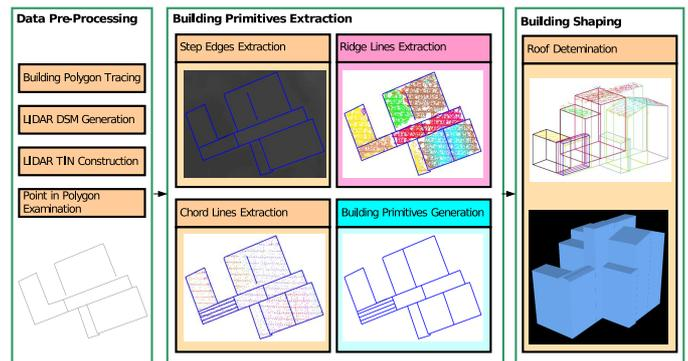
Figure 4. Fusion of LIDAR and vector map for building models.
