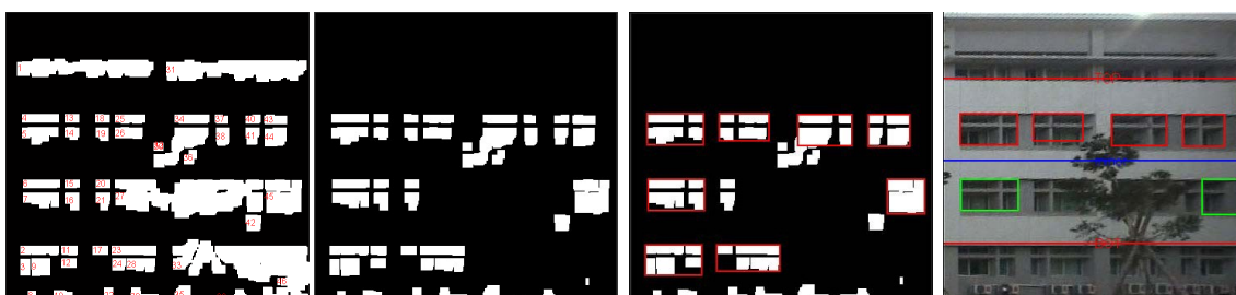
Figure 2: Automatic determination of mirroring axis. From left to right: (a) region-growing segmentation of binary image; (b) identification of possible target areas; (c) homogeneity test to merge segments; (d) calculating the mirroring axis.
